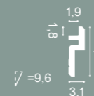
C394 STEPS 200 x 9,5 x 3,1 cm Purotouch® Designed by Orio Tonini
